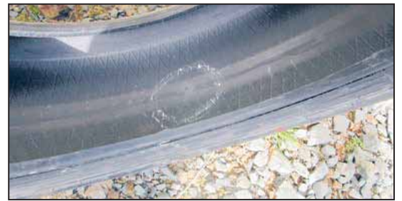
One of the many punctures caused by the coarse hard blue rock spread on Millbrook Rd.
